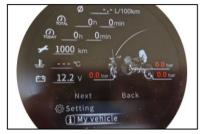
B. Display instrument version information, display software version and hardware version, short press MODE to switch options (previous page or next page), short press SET to confirm;
