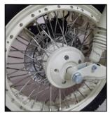
Note\*: Please check the spoke tension after driving 1000Km. If there is any problem, adjust it immediately. Check the spoke tension every 3000Km thereafter.
